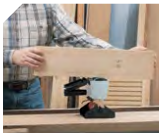
Gluing with the upper roller.
