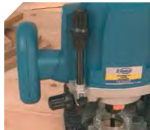
Micrometric adjustment of routing depth. 6 adjustable depth positions for rapid selection of the desired depth.
