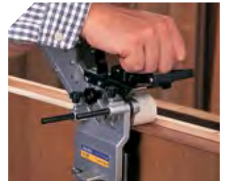
Banding the internal side of a lapped door.
