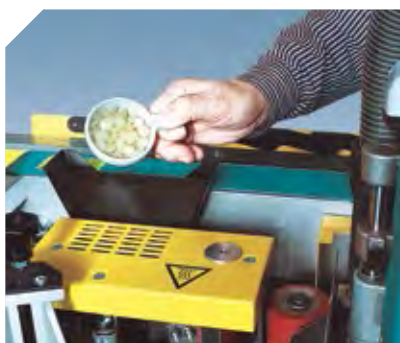
Easy to reload thanks to the special chute. It's equipped with dispenser to reload the glue while working, with no need to stop the machine.
