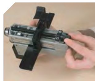
Micrometric regulation of the cutting width.
