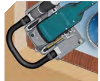
Makes cutting slots in the 4 corners easy. Register on the bevelled front of the reversible base.
