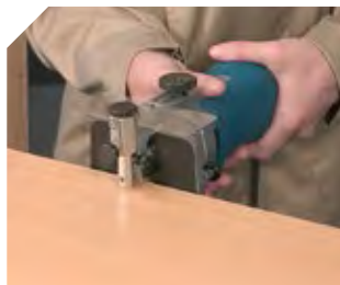
Excellent finishing when trimming laminates.
