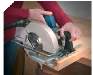
Performs cuts of up to 70 mm.
