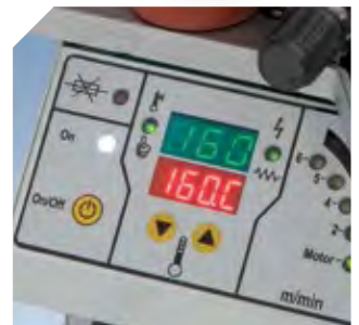
Temperature adjustment (120 to 200°C) controlled by microprocessor for higher accuracy on measurement.
