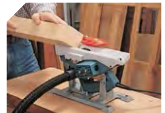
Planer stand for using the planer in a stationary position.
