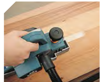
Connection to dust collector with the standard dust collector attachment (optional).
