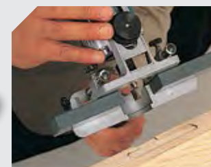
Optional Trimming head for fitting hinges ZB93 (ref. 1750000).
