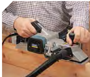
Dust collector connection.
