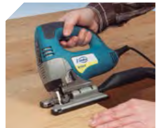
Base can be tilted from 0° to 45°.
