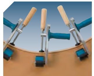
Fixing tapes on concave panels
