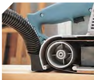
External dust collector connection on model LB31E.
