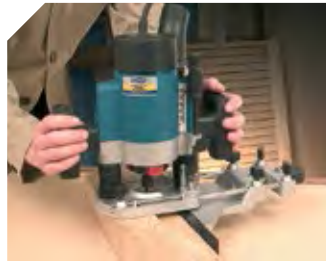
High precision and stability during routing.
