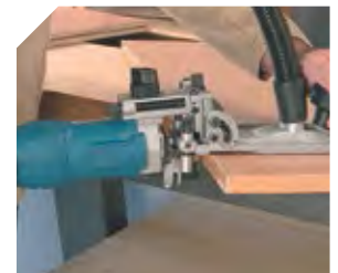
Trimming the edge with the straight bit.
