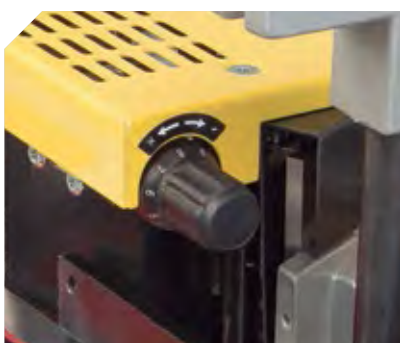
Precise control of the glue dosage on the tape, which helps to adapt correctly the performance of the machine to different kind of materials.
