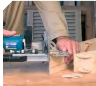
Stronger joints with No. 6 splines.
