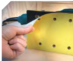
Mobile base for use with velcro sandpapers.
