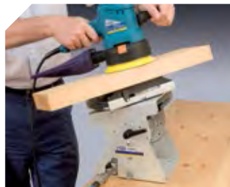
Folding and rotary adjustable support.
