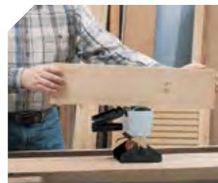
Gluing with the upper roller.
