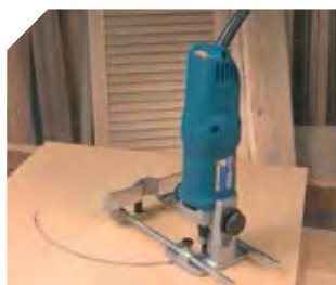
Trimming circular slots.
