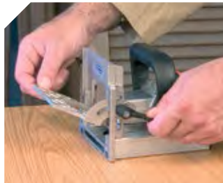
Angle and height of the front fence can be adjusted on a graded scale.
