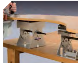
Gripping large pieces with the help of an SVN470 auxiliary unit.
