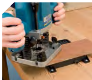
Securing small pieces on a divided portion of the suction plate.
