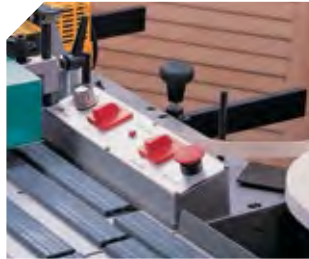
Safety control (STOP). Electronic temperature control.
