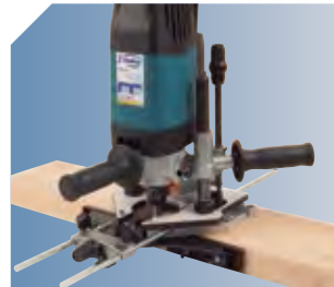
Big support surface for trimming works on edges.
