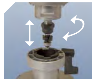
The new fine adjustment system makes it very easy to regulate the trimming head height.
