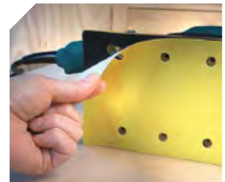
Mobile base for use with velcro sandpapers.
