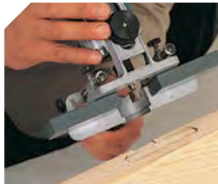
Placing hinges with the ZB93 head.
