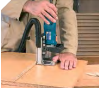
Joints in middle of board.
