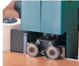
Power trimming unit: trimming both sides simultaneously.
