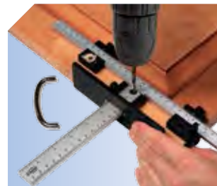
Drilling for door handles.
