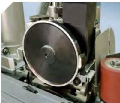
Trimming unit with digital adjustment. Possibility to trim with different radius or 10° chamfer. Excellent finishings without adhesive residue due to the double flat scraper. Automatic front and rear flush cutting.
