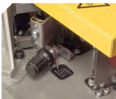
Simple and fast tape thickness adjustment. It allows tapes up to 3 mm thick.
