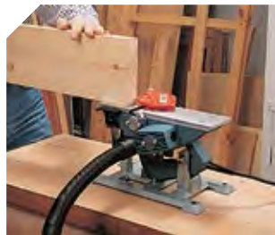
Planer stand. To be fixed to a workbench for using the planer in a stationary position.
