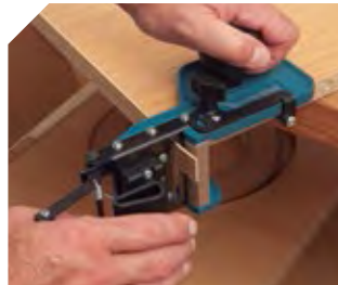
Cutting on both sides on straight panels.
